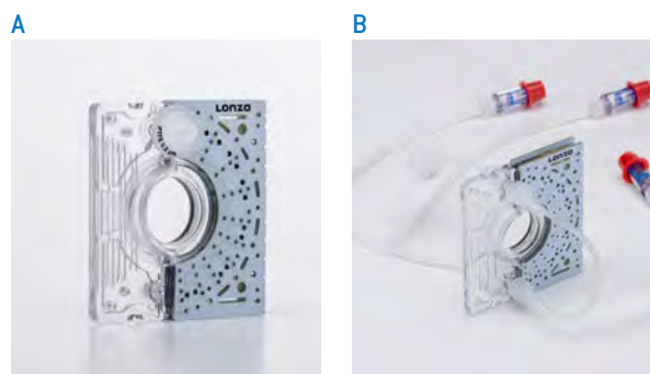
Two formats available. [A] 1 mL Nucleocuvette™ Cartridge: 1 mL filling volume for up to 1 \times 10^9 cells (manual filling via sterile injection port) [B] LV Nucleocuvette™ Cartridge: Up to 20 mL processing volume (in 1 mL steps) for up to 1 \times 10^9 cells (automatic filling via reservoirs or bags)
